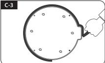
Remove friction tape and allow to dry
