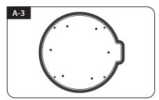
Attach friction tape outside of the mounting plate by 5mm away from the plate edges
