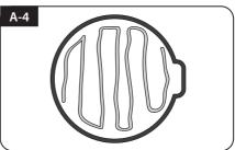
Put aside the mounting plate to apply silicone within the attached tape line but leave 2cm inward gap from the line
