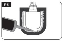
Apply silicone around cable holder and on the top of the screws for waterproof
