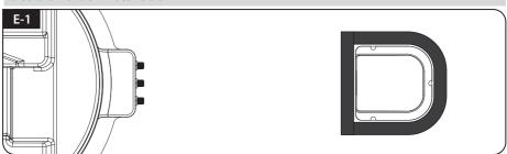
Place cable holder around 30CM from the rear centre of the antenna. Apply friction tape 5mm from the outside of the holder
