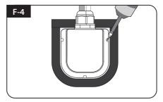
Fix cable holder on the vehicle roof with three(3) of M4 x 20 screws at drill holes made
