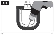
Place the assemble cable holder inside the tape markings. Drill three(3) 2mm holes
