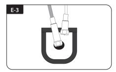
Make sure that hole size is big enough to insert all cables together by one and one
