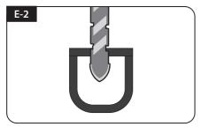
Drill a 20mm hole (or larger) in the centre of the tape marking
