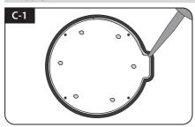
Apply silicone around mounting plate edge
