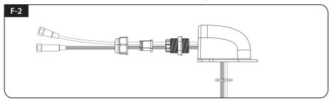
Put the cable inside the Cable holder as above picture.
