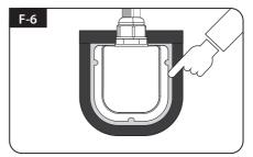
Connect cables to relative ports. Remove friction tape then tidy silicone before dry
