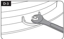
Fit the supplied nuts to each of the four bolts and tighten firmly with spanner
