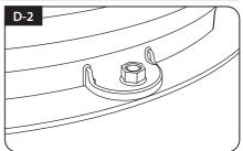
Place the antenna on the aluminium plate and place the washers over each bolt
